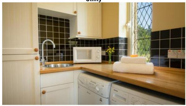
height of worktop is 930mm depth of worktop is 600mm minimum clearance is 800 mm light switch is 1160mm from ground floor
