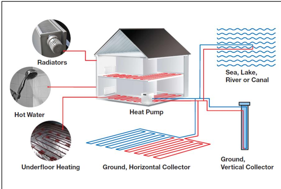
Figure 1: How a heat pump works. Diagram courtesy of the Ground Source Heat Pump Association (GSHPA)
